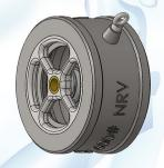
A full range of surge reduction (non slam or nozzle) check valves reduces the effect of water hammer in a pumping system.
