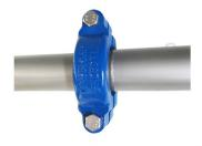
The couplings are supplied with hubs prepared for standard butt welding to all pipes. The hubs create the pipes' engagement when brought together by the clamps. The taper angle, combined with smoothed taper surfaces, enable a powerful engagement force with minimum required bolting torque. The HMP™\_TE tapered coupling idea comes from the T&E (Trucking and Engineering / Robor) T&E coupling, that was re-engineered and improved upon. The coupling is fully interchangeable with the T&E coupling
